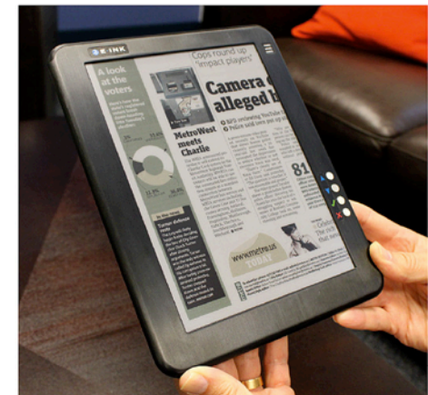
(d) E Ink Vizplex film applied to rollable (Polymer Vision) demonstrators and photograph of the new E Ink color demonstrator
