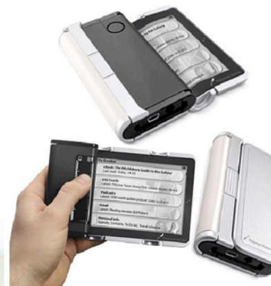
(d) E Ink Vizplex film applied to rollable (Polymer Vision) demonstrators and photograph of the new E Ink color demonstrator
